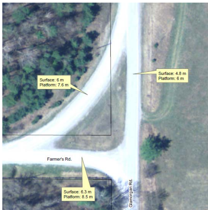
Figure 2. Measurements showing narrow Glamorgan leg.
