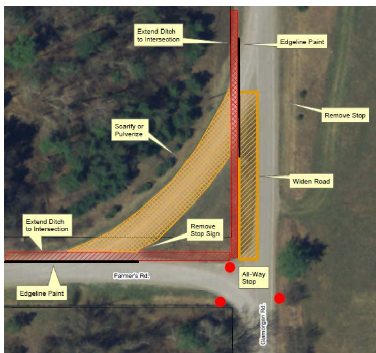
Figure 4. Showing curve closure, leg widening and all-way stop.
