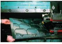
A surviving pressed metal shingle was used as a prototype for manufacturing replacement shingles when restoring the main house at the Motherwell Homestead near Abernathy, SK. In Restoration, repairs or replacements of extensively deteriorated or missing parts of features are done in kind, and are based on physical, documentary and oral evidence.
