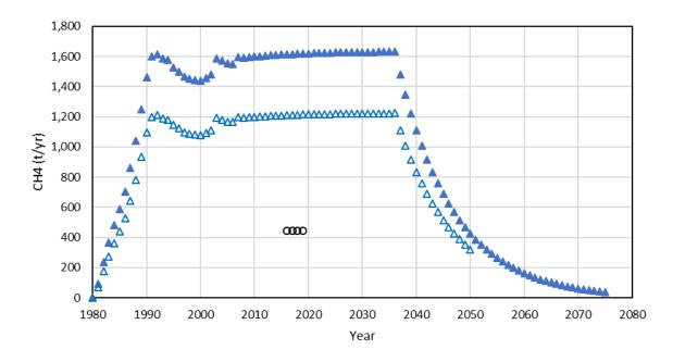
Figure 18 - Predicted Methane Generation Rate (Golder, 2008)
