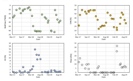
Figure 3 - Summarized Monitoring Results for GW3-H
