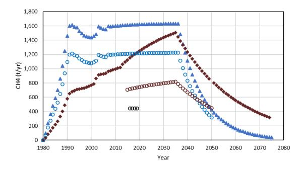
Figure 19 - Predicted Methane Generation Rate (Golder, 2008)
