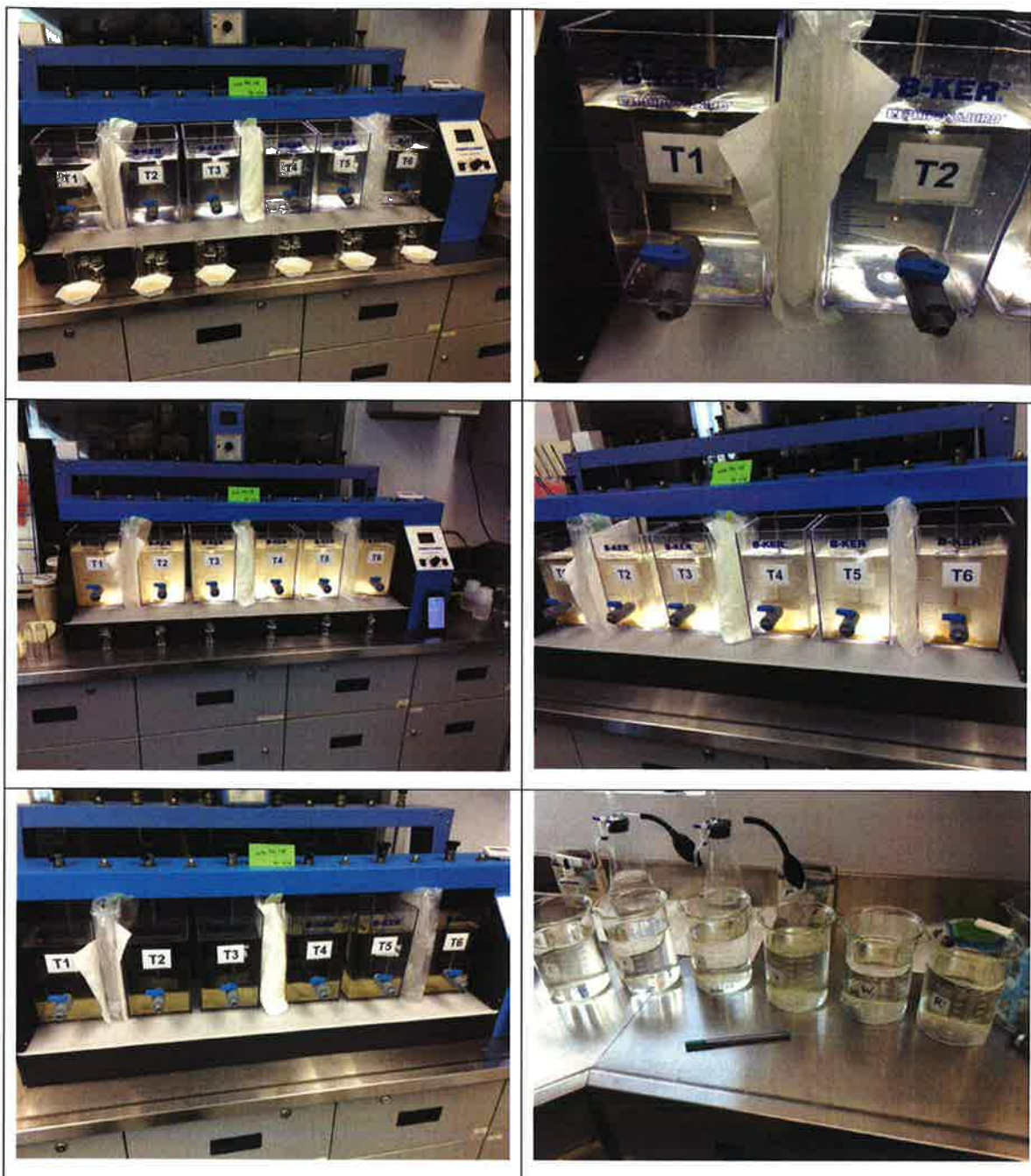
Figure 4 Time Lapse of Jar Test for one coagulant
