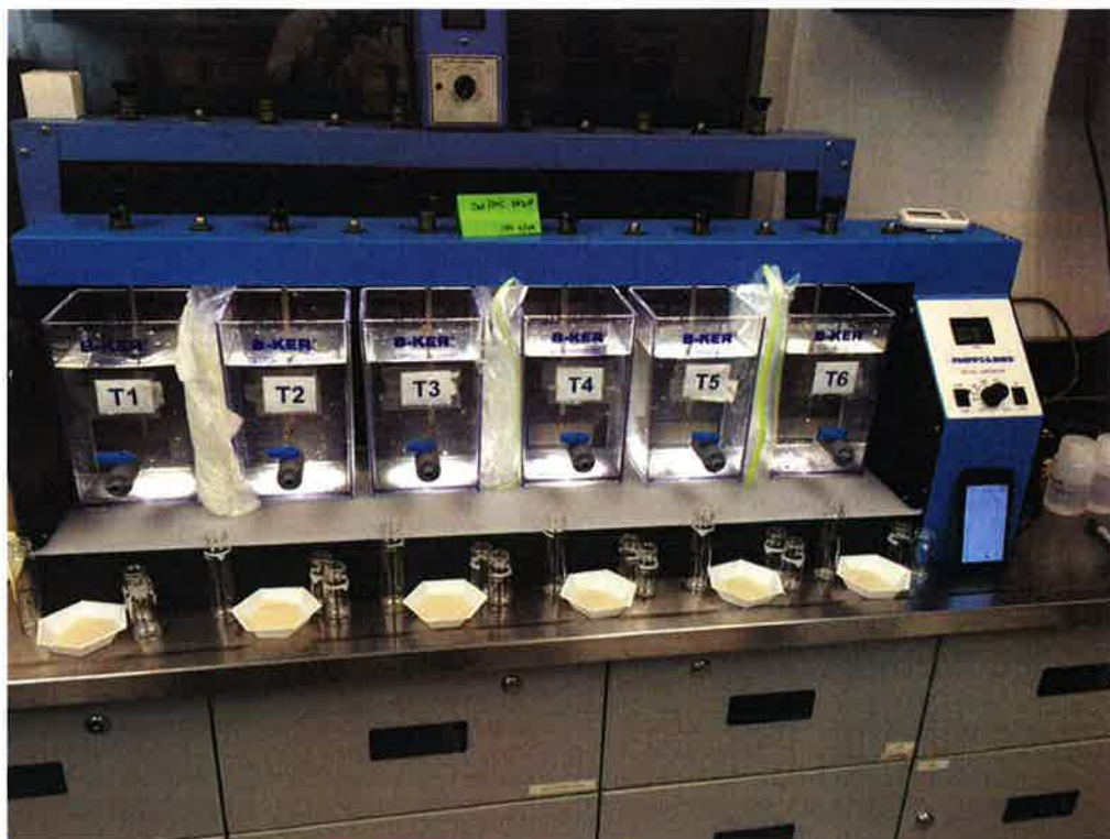
Figure 1 Jar Testing Apparatus used for testing the coagulants
