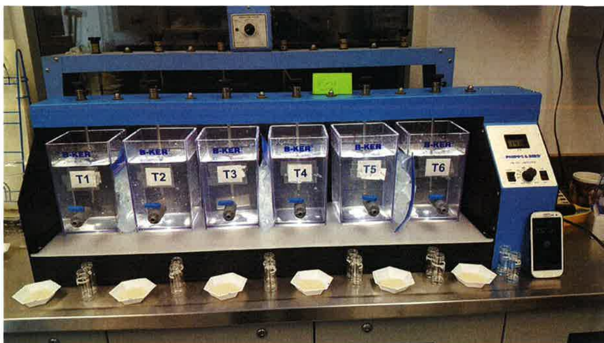
Figure 1 Jar Testing Apparatus used for testing the coagulants
