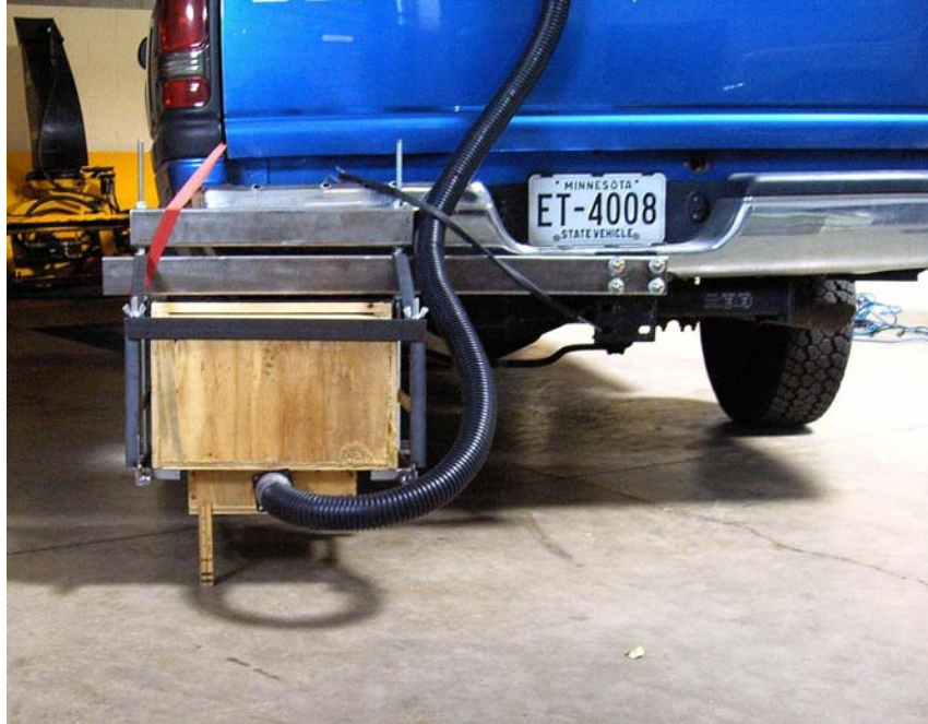
Figure 2 Ground clearance for hitch-mounted dust collection gear.
