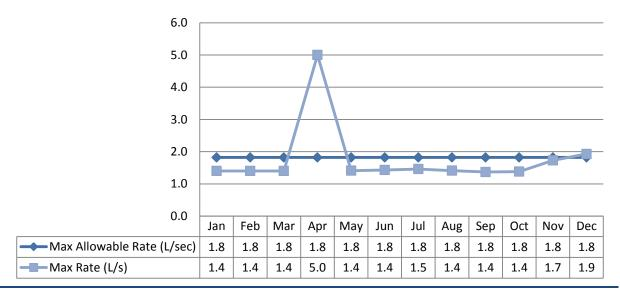
Note: The above table shows there was an exceedance in instantaneous peak flow rate (L/s) in December. This exceedance was short in duration. The significant spike in April was due to scheduled Flow Meter calibration.
