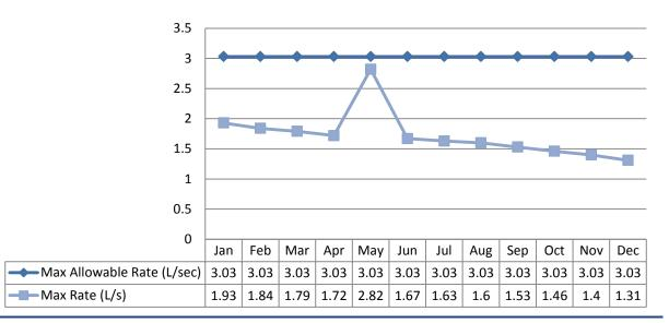
**Note:** The above table shows there were exceedances in instantaneous peak flow rate (L/s). The significant spike in May was due to scheduled Flow meter calibration.
