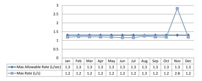
Note: The above table shows there were exceedances in instantaneous peak flow rate (L/s). The significant spike in November was due to scheduled Flow Meter calibration.
