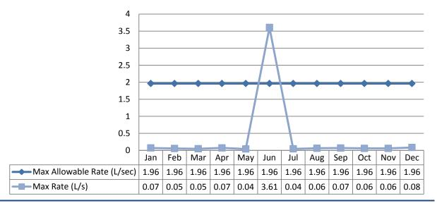
**Note:** The above table shows there were exceedances in instantaneous peak flow rate (L/s). The significant spike in June was due to scheduled well cleaning.
