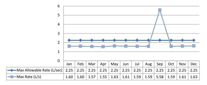
Note: The above table shows there was an exceedance in instantaneous peak flow rate (L/s). The significant spike in September was due to scheduled Flow Meter calibration.
