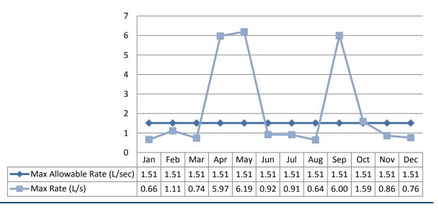
Note: The above table shows there were exceedances in instantaneous peak flow rate (L/s) this is due to well pump start-up. Additionally, in September the Flow Meter was scheduled for calibration.
