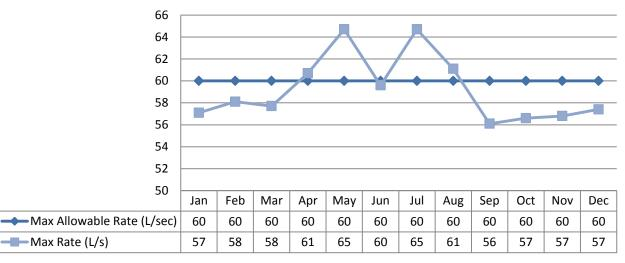
Note: The above table shows there were exceedances in instantaneous peak flow rate (L/s) which were short in duration. The scheduled Flow Meter calibration was in July.
