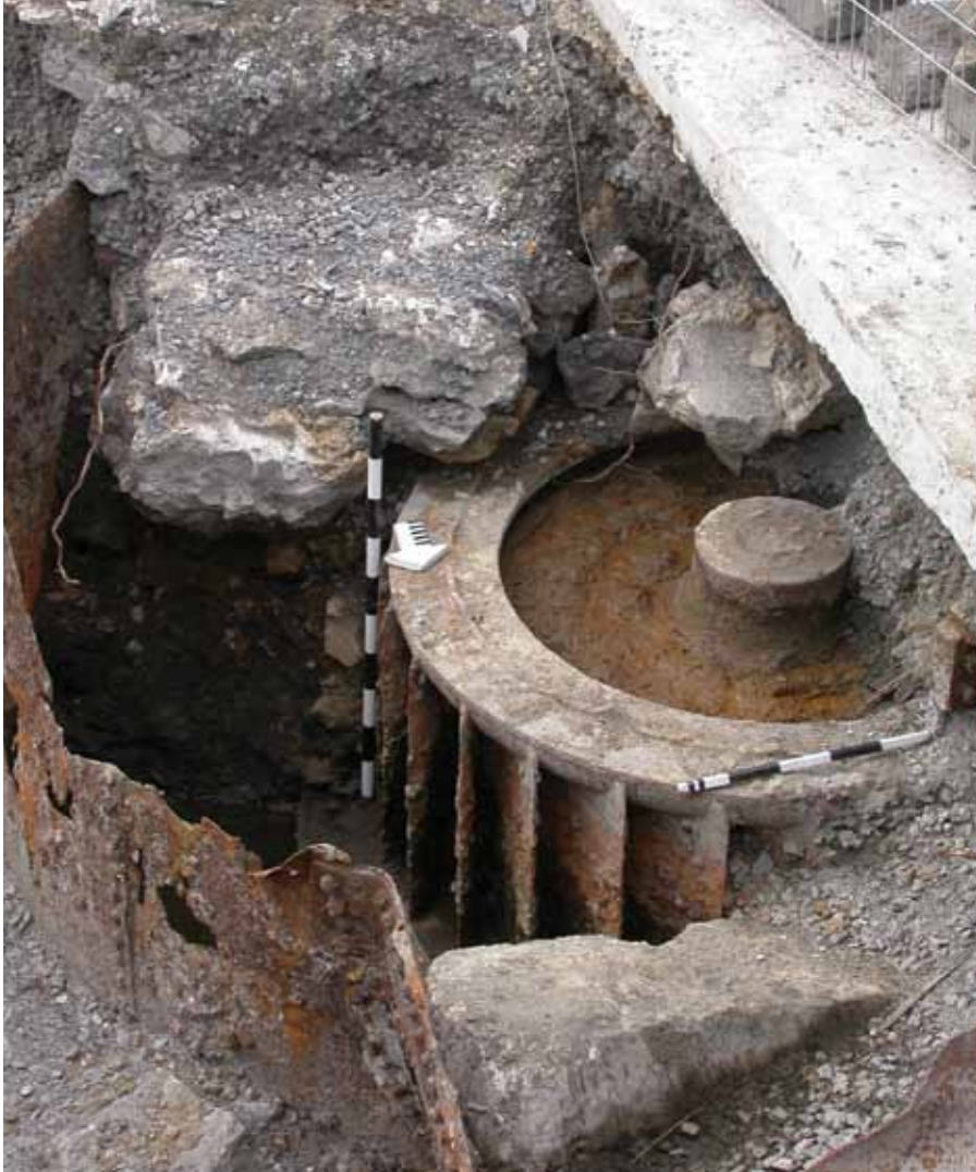
This partially uncovered hydraulic turbine at Pointe-des-Seigneurs, Lachine Canal National Historic Site of Canada in Montreal was installed and used by the Caledonian Iron Works Co. in the late 19 th century.
