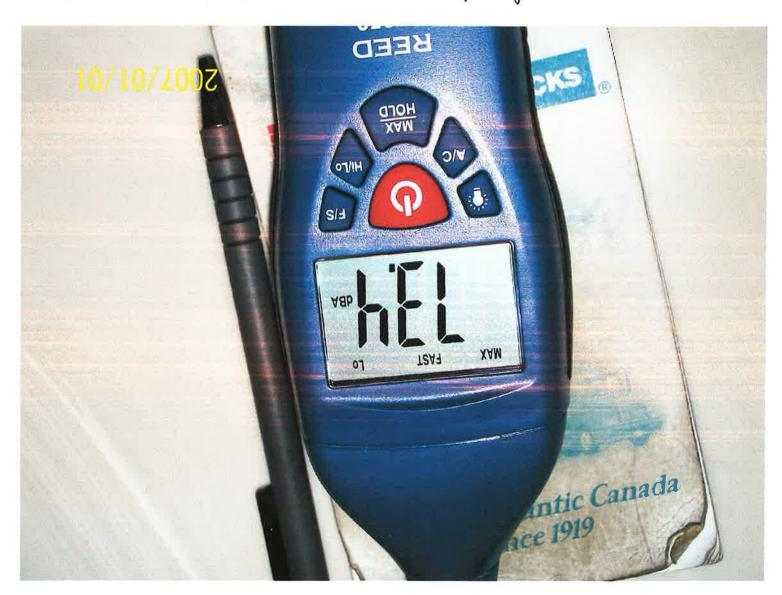
This is a desiber meter which is roading the moster cycle on the moise bush of a measurement in my Carrection roading this measurement in my personation room with all doors and windown
