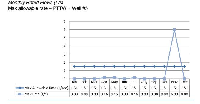
**Note:** The above table shows there were exceedances in instantaneous peak flow rate (L/s). The significant spike in November was due to scheduled Flow Meter calibration. Well 5 was taken out of service June 2022 and returned to service December 6 2023, but not in production rotation.
