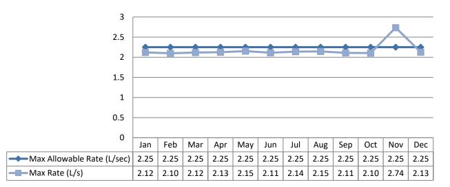
Note: The above table shows there was an exceedance in instantaneous peak flow rate (L/s). The significant spike in November was due to scheduled Flow Meter calibration.
