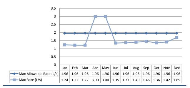
Note: The above table shows there were exceedances in instantaneous peak flow rate (L/s) but these exceedances were short in duration. Spikes recorded by on-line instrumentation were a result of air bubbles and various maintenance/calibration activities. The significant spike in May was due to scheduled Flow Meter calibration. All spikes are reviewed for compliance with O. Reg.170/03.
