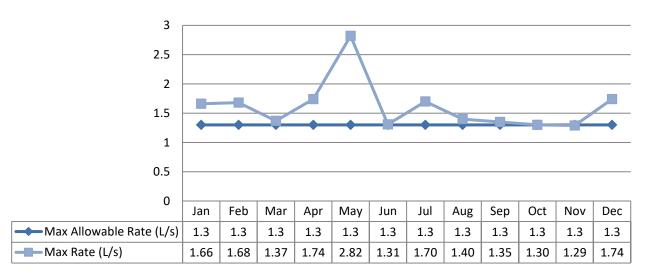
Note: The above table shows there were exceedances in instantaneous peak flow rate (L/s) but these exceedances were short in duration. Spikes recorded by on-line instrumentation were a result of air bubbles and various maintenance/calibration activities. The significant spike in May was due to schedule flow meter calibration. All spikes are reviewed for compliance with O. Reg. 170/03.
