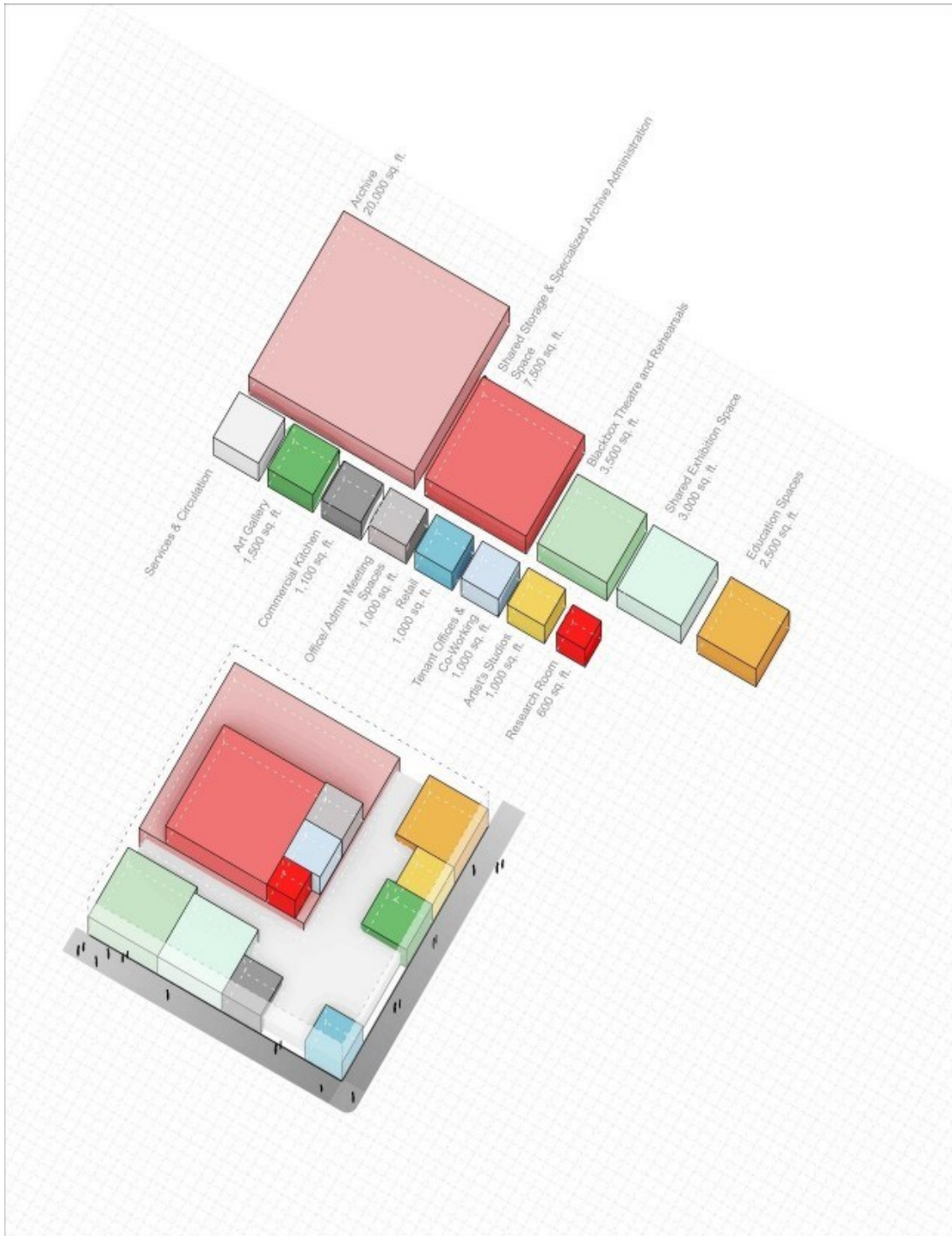
Figure 5.1: Programming Diagram for the City of Kawartha Lakes Culture Centre At top, the programs are shown as blocks indicating their size in relation to one another. The diagram shows their relationship with each other, as well as a street frontage. It should be noted that the diagram is not intended to reflect a specific site.
