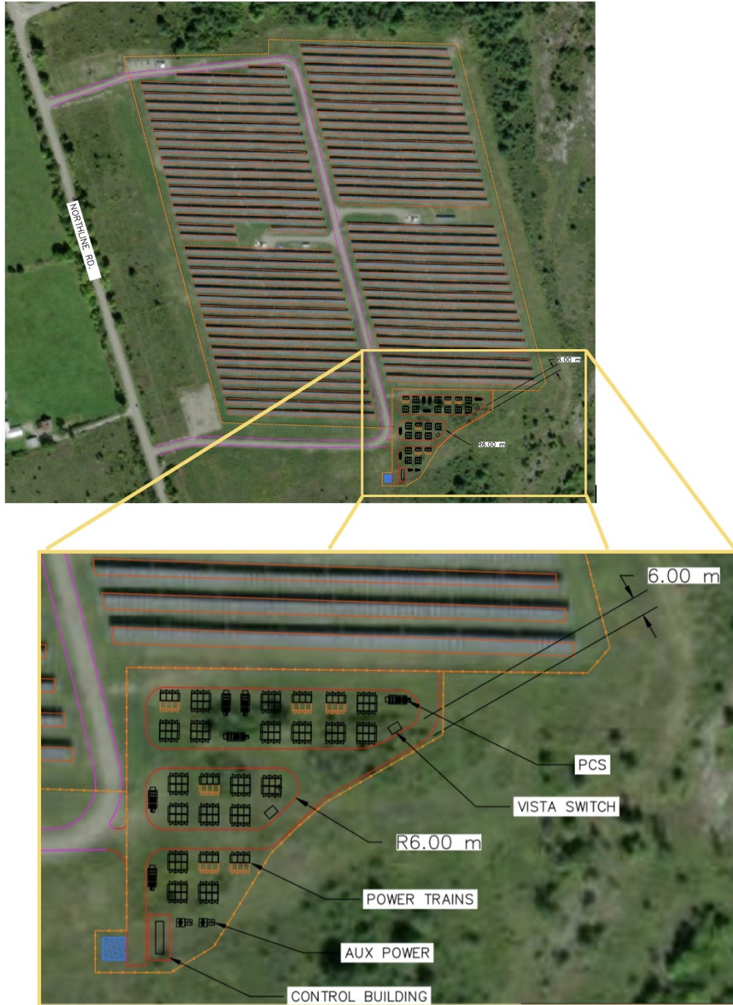
Figure 3: BESS site layout
