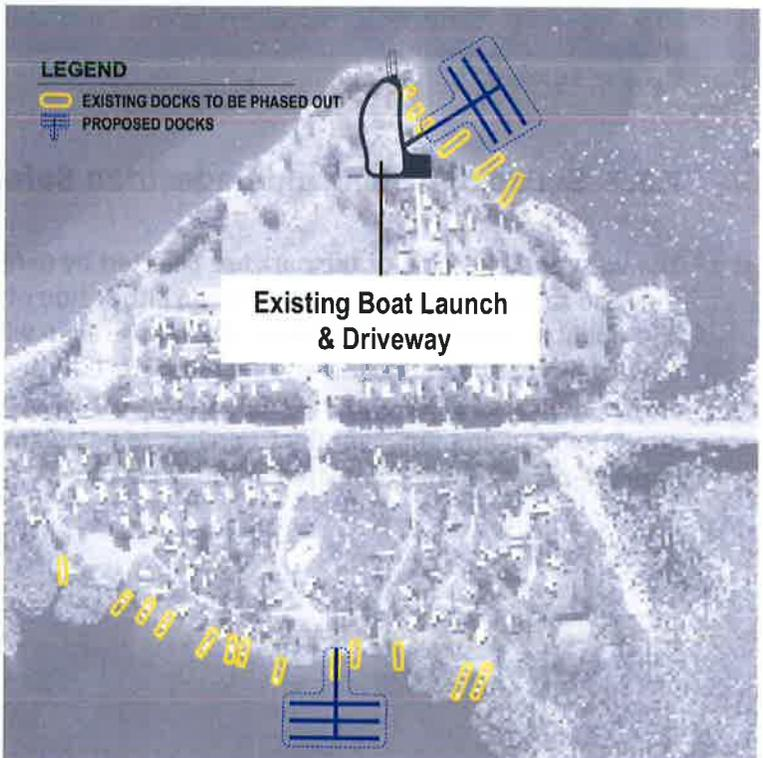
Figure 34: New centralized docks, docks to be phased out, and location of existing boat launch
